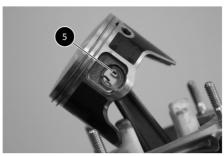
Make sure the piston is in the right way: the arrow engraved on its crown must point towards the exhaust port.
