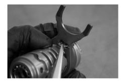
• - Place the clip so that the right hand side passes through the left hand hole to hold the guide pin and then lock the clip through the right hand hole.
