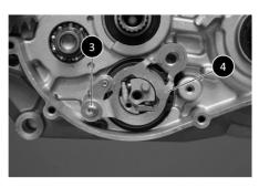
• Fit the screw 5 and tighten it to a 20Nm torque, tighten the screw 3 to a 7Nm torque, fit the holding plate and tighten the screw 6 to a 5Nm torque.
