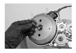
Using the flywheel puller <u>part number 10984</u>, remove the flywheel.
