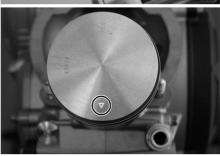
Make sure the rings ends face the piston pins.
