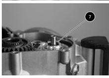
Remove coolant pump snap ring
