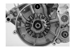
• Fit the CHC screws **5** and the screw **6** with the wiring holding plate.
