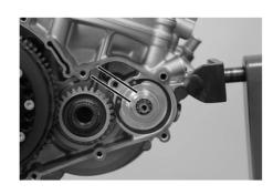
• Fit the drive pin **22** in the water pump's shaft.
