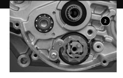
Install the secondary shaft's snap ring
