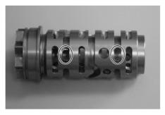
Using a pin driver, push the pin to the inside of the drum.
