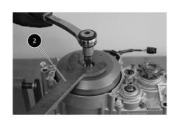
• Put the flywheel puller tool's extension <u>part</u> <u>number10984</u>.
