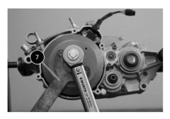
• Fit the ignition cover then tighten its four screws at a **8Nm** torque.
