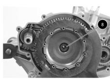
• Remove the needle cage **9**, and the clutch basket **10**.
