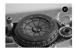
Fit the diaphragm spring 18 and its centering tool
