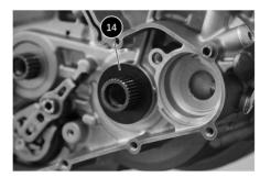
Remove the snap ring from the crankshaft
