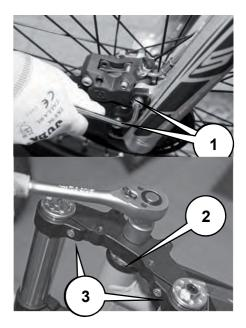
Undo the steering stem counternut, 4 and its dust cover, then remove the fork from the frame.
