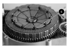
ullet Remove the clutch pusher  $oldsymbol{0}$  , and the pushrod
