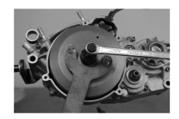
Remove the 3 stator screws
