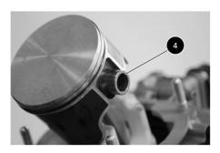
• Fit the clips on both sides of the piston **5**.
