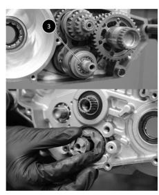
To withdraw the gearbox, you must remove all the components ( shifting drum, primary and secondary shafts ) in one batch. If needed, slightly hit the shafts with a rubber mallet.
