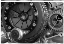
Fit the water pump, then its snap ring. Make sure the ring end gap is lined up towards the pump gear's shaft hole.
