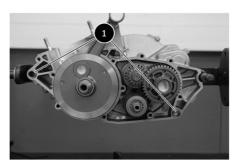
• Fit the nine screws ② , with a copper washer under the screw ③ Tighten them to a 10Nm torque.
