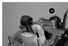
tilt the inlay to the rear and remove it to the top.
