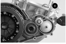
Remove idle gear shaft
