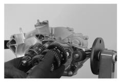
Install the shifting drum's snap ring and remove the shifting locator locking tool.
