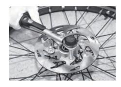
Reassemble the wheel following the reverse procedure, applying a thin coat of grease on the front wheel spindle.
