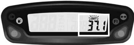
Fig 6 Adjustable trip distance function
