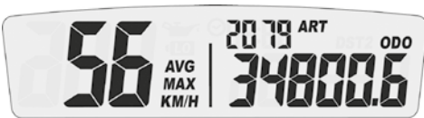
Screen 3: Alternating AVG/MAX speed, Accumulated run time, ODO
