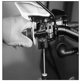
Remove original main standard lighting sub harness P/No.8145 and replace with the racing lighting sub harness.6845.
