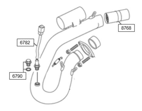
Fit the lambda sensor cap connector provided with the motorcycle
