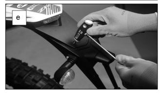
Remove original speedo holder (4389) and replace with racing speedo bracket 4526
