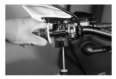
Remove original main standard lighting sub harness P/No.8145 and replace with the racing lighting sub harness.6845.
