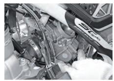
Dismantle the fuel input tube. Open the upper cap and remove the sliding hood. This leaves the carburettor completely unfastened.
