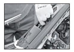
Loosen and remove the filter box's fastening screws as well as those of the rear mudguard.
