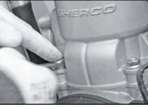
Lubricate the ends of the connecting rod and the roller bearings.
