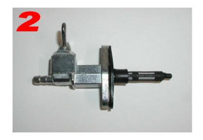
View of the fuel valve after it has been removed from the fuel tank.
