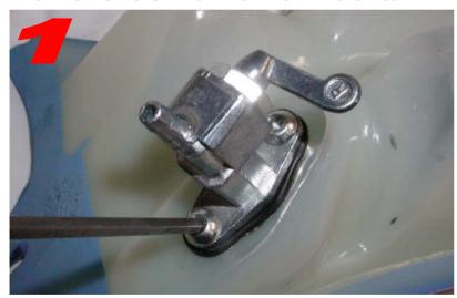
Using a 4mm "ball" end Allen wrench, remove the fuel valve from the fuel tank.
