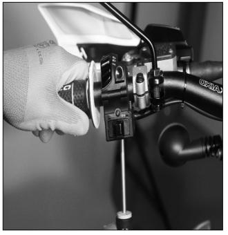
Remove original main standard lighting sub harness P/No.4388 and replace with the racing lighting sub harness.6845.
