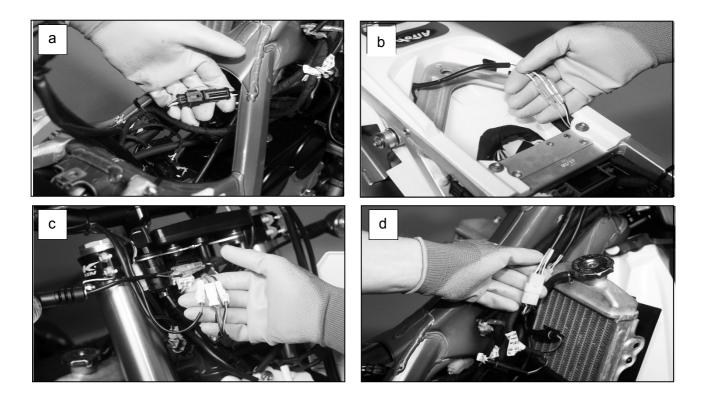
Remove original accessory wiring sub harness (3509) and start disconnect:
