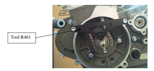
➤ Install the camshaft with the cam lobes downward. The marks on the drive gear should align with the valve cover mounting surface.
