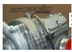
Install the rubber antivibration block on the oil supply tube as shown
