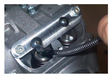
❖ <u>Note</u>: To determine the thickness of the shim required, measure the shim and subtract 2mm.
