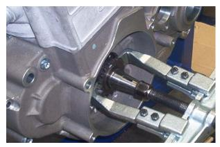
■ **NOTE**: To remove the cam chain use tool #R463.
