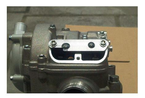
> Rotate the engine in the opposite direction to release the shims.
