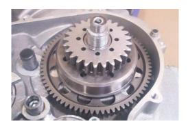
Apply thread locking material to the threads, install the crankshaft nut and tighten to **150 Nm**.
