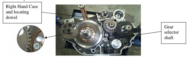
• Install the Left Hand Case. Tap with a nylon hammer if necessary. Tighten the screws to **11Nm.**
