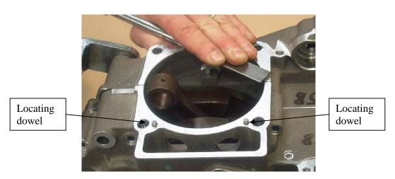
Install the two cylinder locating dowels; using tool #R454 (Photo 1) install one of the circlips in the groove in the piston (Photo 2), lubricate the piston pin and install it in the piston and the connecting rod, again using tool #R454 install the remaining circlip.
