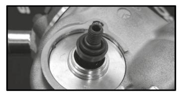
· Remove the lids from each side of the valve
