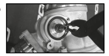
• Remove the O-ring and pulley spacer.
