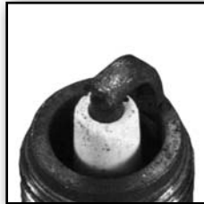
Spark plug has dry deposits
