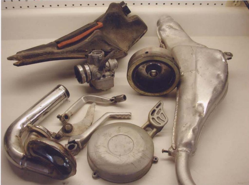
Leave bolts in brake pedal, shift lever, and silencer. Place flywheel/crankshaft Woodruff Key inside magnetic flywheel for safe storage until reassembly
