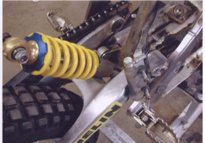
After engine removal with swingarm pulled back.
