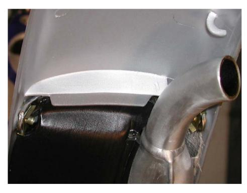
This picture shows the fender to air box joint before sealing.
