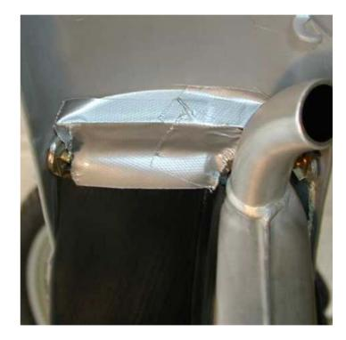
This picture shows the joint sealed with duct tape. Weather stripping can also be used.
